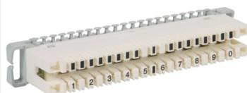
Type 2 for LSA technology for connecting 10 pairs each on the cable and routing side. Protection is provided between the disconnection contacts as soon as DRL components are plugged in. DPL 10 G3 arresters can also be plugged into the disconnection block.
