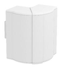
External corner cover made of halogen-free PC/ABS for changing the direction of Rapid 80 device installation trunking of the GK, GKH, GS and GA systems. The fittings can be variably adjusted between 80° and 100° and can be used in symmetrical and asymmetrical trunking.
