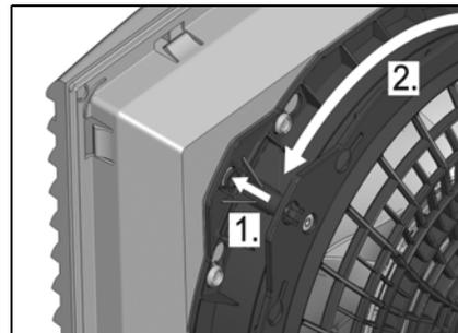
Fig. 5: Release the bayonet connection
