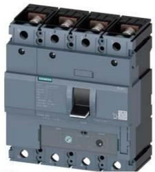
CIRCUIT BREAKER 3VA1 IEC FRAME 250 BREAKING CAPACITY CLASS M ICU=55KA @ 415 V 4-POLE, LINE PROTECTION TM240, ATAM, IN=250A OVERLOAD PROTECTION IR=175A ...250A SHORT CIRCUIT PROTECTION II=5...10 X IN NEUTRAL PROTECTION 1 BUSBAR CONNECTION
