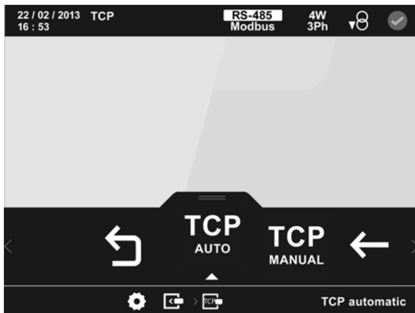
Figure 217: Main configuration screen of the Modbus TCP communications module.
