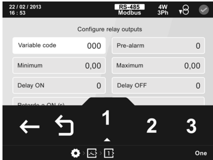
Figure 130: Configuration screen of relay digital outputs.
