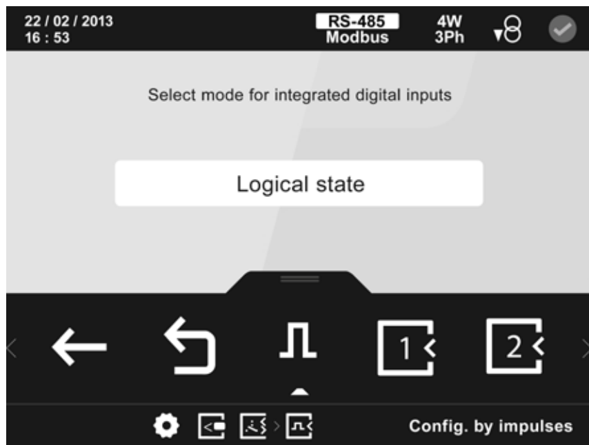
Figure 157: Main configuration screen for relay digital inputs.
