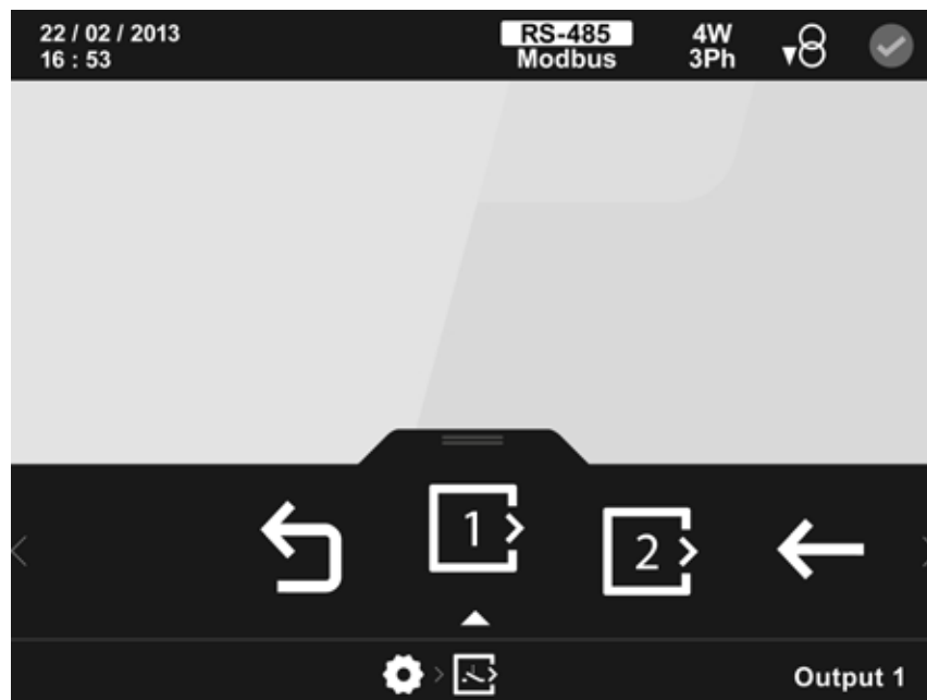
Figure 129: Main configuration screen of relay digital outputs.
