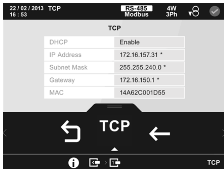
Figure 110: Information screen of the Modbus TCP ( Switch ) module (TCP communications).
