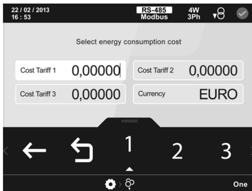
Figure 125: Energy consumption costs configuration screen.
