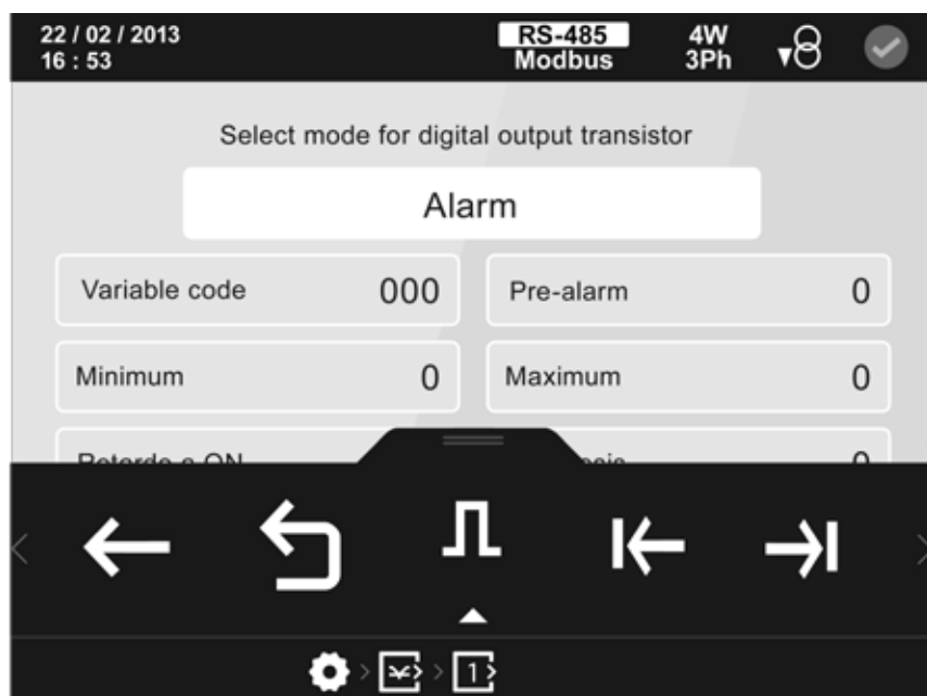
Figure 132: Configuration screen of transistor digital outputs (alarm mode).
