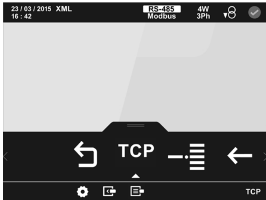
Figure 209: Main configuration screen of the Datalogger module.
