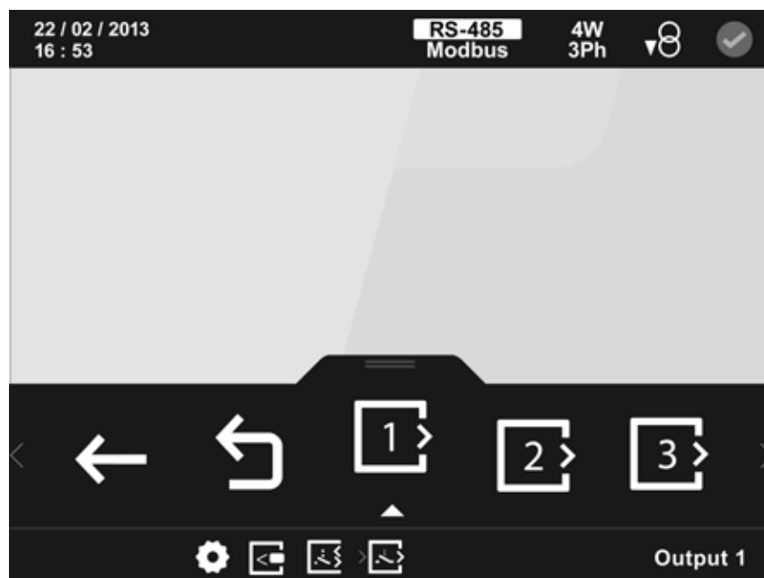
Figure 158: Main configuration screen of relay digital outputs.
