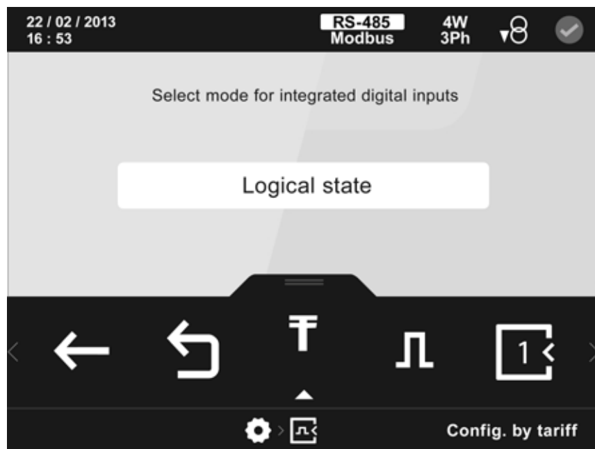
Figure 134: Main configuration screen for digital inputs.
