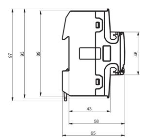
B24 The following drawing shows the physical dimensions of the B24 meters.
