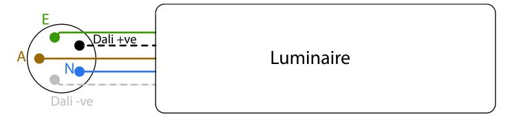
Note for non-dimming versions of the Product: the Dali +ve, and -ve cables are redundant and do not need to be connected.
