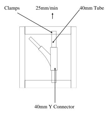
Connect three pieces of 40mm duct. Ensure all the connections are tightened. Place the assembly in a tensometer connecting the two 63mm tubes to the opposing jaws and perform a destructive test at a rate of extension of 25mm/minute.
