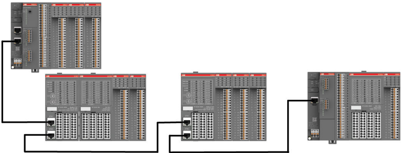
Fig. 4: I/O modules (S500-eCo) connected to an AC500-eCo processor module via Modbus/TCP network, using a Modbus/TCP communication interface module or a processor module as client.
