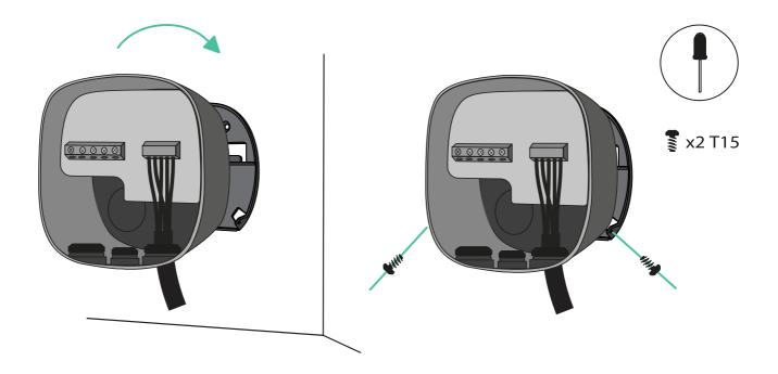
Make an incision on the grommet and insert the power supply cable.
