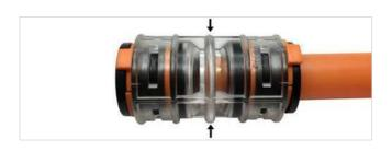
Make sure that the Microduct is correctly and fully inserted. The transparent body of the Connector allows a visual inspection of the correct and full insertion of the Microduct. Insertion of the Microduct into the Connector requires a moderate force. The Microduct and the Connector seal should not be scratched or damaged during the insertion, otherwise there may be leaks or further mis-functioning. Please, connect the Microduct by hand, without using any kind of tool.
