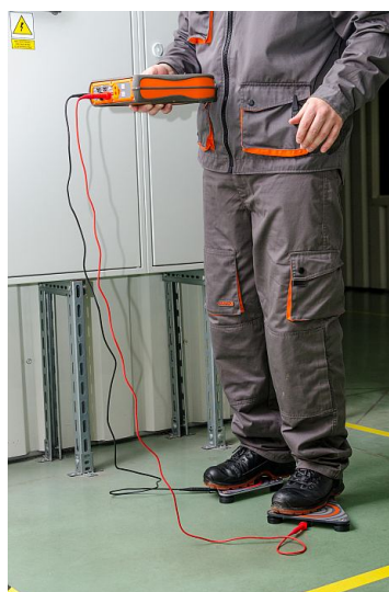
Fig. 4. Surface resistance measurements using two PRS-1 test probes.
