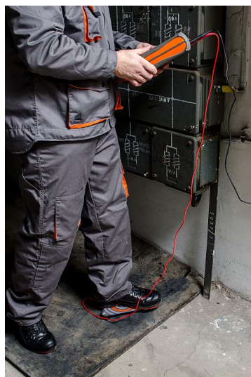
Fig. 3. Resistance measurement on floor or wall with the PE conductor in use.
