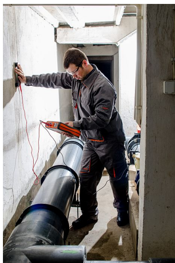
Fig. 3. Resistance measurement on floor or wall with the PE conductor in use.
