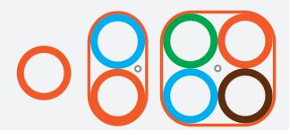
Höhle microducts are designed for long term protection of fiber optical cables. Direct Bury (DB) type of microducts are thick wall products that attain their mechanical robustness and functional performance through their intrinsic thick walls and need no further protection at underground installations. Höhle microducts conform to BS FN 61386 and BS FN 60794-5.
