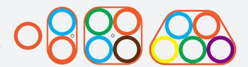
Höhle microducts are designed for long term protection of fiber optical cables. Direct Bury (DB) type of microducts are thick wall products that attain their mechanical robustness and functional performance through their intrinsic thick walls and need no further protection at underground installations.
