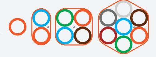
Höhle microducts are designed for long term protection of fiber optical cables. Direct Bury (DB) type of microducts are thick wall products that attain their mechanical robustness and functional performance through their intrinsic thick walls and need no further protection at underground installations. Höhle microducts conform to BS FN 61386 and BS FN 60794-5.
