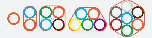
Höhle microducts are designed for long term protection of fiber optical cables. Direct Install (DI) type of microducts are thin-walled products designed to be installed into a conduit that provides the primary mechanical protection for innerduct and cable pathway.
