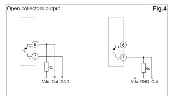
The load resistance (Rc) must be designed so that the closed contact current is under 100 mA ( $V_{\rm on}$  is equal to 1 V dc). DC voltage ( $V_{\rm off}$ ) must be less than or equal to 80 V.
