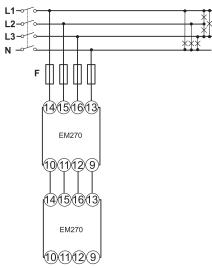
**Fig. 9** Example of connection of multiple EM270s in cascade.
