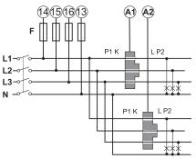
**Fig. 6** Three-phase system, three single-phase circuits.
