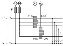
**Fig. 8** One-phase system, six single-phase circuits.
