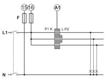
**Fig. 7** One-phase system, three single-phase circuits.
