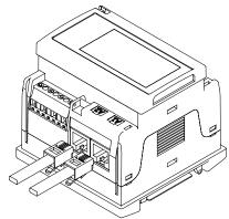
Fig. 19 RJ11 connections
