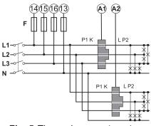
**Fig. 3** Three-phase system, one three-phase circuit.
