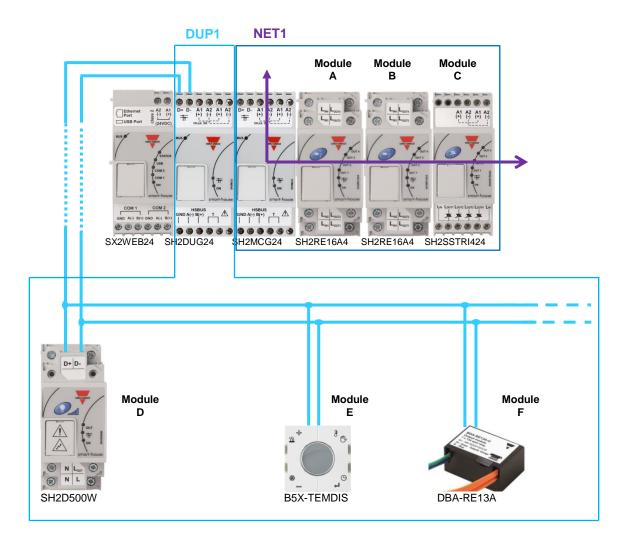
Modules A, B, and C are connected to the smart Dupline network (NET1).
