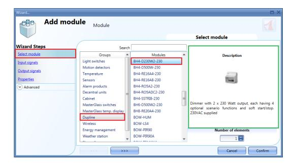
The user must be sure to assign the correct network to the BH4-D230W2-230 in the software, according to the network the BH4-D10V2-230 is connected to.
