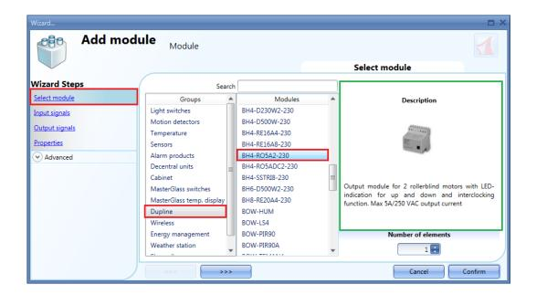
The user must be sure to assign the correct network to the BH4-RO5A2-230 according to the network the BDC-RO5A-230 is connected to.
