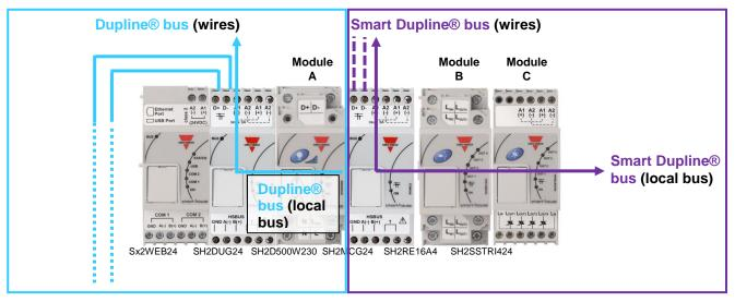
Module **A** is connected to the Dupline® network **1** (SH2DUG24 Dupline network).
