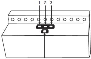
The bus extension module connected to the #1 socket on the controller is identified as Bus 1, the bus extension module connected to the #2 socket on the controller is identified as Bus 2 and the bus extension module connected to the #3 socket is identified as Bus 3.
