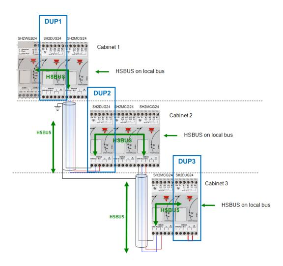
Like the other bus generators, each SH2DUG24 has an SIN address that has to be programmed using the Sx tool.
