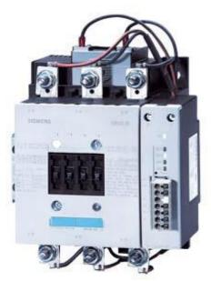
CONTACTOR, 55KW/400V/AC-3 AC(50...60HZ)/DC OPERATION UC 96-127V AUXILIARY CONTACTS 1NO+1NC 3-POLE, SIZE S6 BAR CONNECTIONS ELECTRONIC OPERATING MECHANISM WITH PLC/SIMOCODE INTERFACE AND REMAIN. LIFETIME INDICATOR
