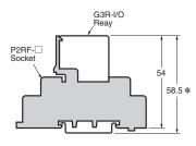
\* These are values when using the DIN track PFP- $\square$ N. Heights become higher by approximately 9 mm when using PFP-□N2.
