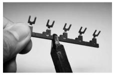
When using a cut short-circuit bar (P2DN), always use the provided cap to protect the charger part.
