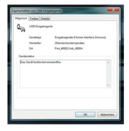
After the installation process is finished successfully you can find the entry under the node HID (Human Interface Devices) in the device manager.
