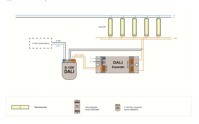
64 DALI-devices controlled by a 0-10V control device using a 0-10V to DALI converter (Art.Nr: 86458352)
