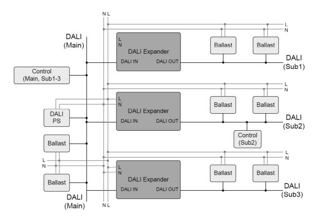
Expansion of a DALI circuit (Main) with multiple broadcast controllable DALI sub-circuits. The additional control module in DALI (Sub2) enables the specific control of the sub-circuit.
