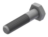
Additional information: Recommended length of the Bolt for U-21 channels is 25 mm when mounting parts with material thickness 5 mm. Recommended length of the Bolt for U-41 channels is 30 mm when mounting parts with material thickness of 5 mm. Increase the length of the Bolt accordingly when mounting parts with more than 5 mm material thickness. Longer lengths in DIN 931 partly threaded. STD: 100
