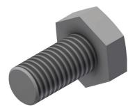
Additional information: Recommended length of the Bolt for U-21 channels is 25 mm when mounting parts with material thickness 5 mm. Recommended length of the Bolt for U-41 channels is 30 mm when mounting parts with material thickness of 5 mm. Increase the length of the Bolt accordingly when mounting parts with more than 5 mm material thickness. Longer lengths in DIN 931 partly threaded. STD: 100
