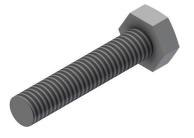
Additional information: Recommended length of the Bolt for U-21 channels is 25 mm when mounting parts with material thickness 5 mm. Recommended length of the Bolt for U-41 channels is 30 mm when mounting parts with material thickness of 5 mm. Increase the length of the Bolt accordingly when mounting parts with more than 5 mm material thickness. Longer lengths in DIN 931 partly threaded. STD: 200
