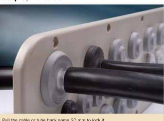
Pull the cable or tube back some 20 mm to lock it.
