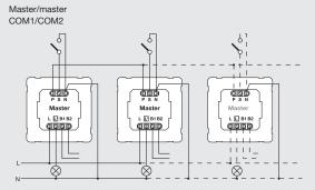
Detector connected to staircase lighting time switch
