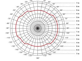
Presence Control PRO HF 360, installation height 2.80 m red = radially
