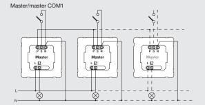
2 detectors connected to external staircase lighting time switch Old building/refurbishment project
