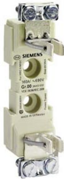
LV HRC FUSE BASDE, 690V(1000V) SINGLE-POLE, 160A, SIZE 00 CLIP-TYPE TERMINAL, 6X70SQMM
