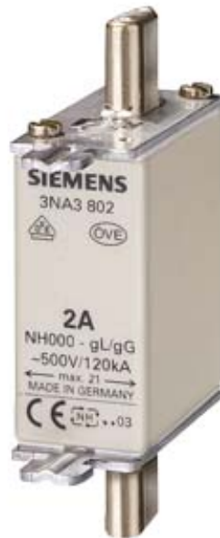
LV HRC FUSE LINK GL/GG WITH NON-INSULATED GRIP LUGS WITH FRONT INDICATOR SIZE 000, 2A, AC 500V/DC 250V
