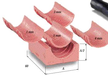
There are nine AddBlocks and together they cover 45 pipe or cable dimensions. The length is always 60 mm and the width of the base block is 20, 30, 40 or 60 mm.
